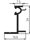
Door Rebate Profile White Art. No. 260008/001 Brown Art. No. 260008/002 (For use with Composite Door Panels)
