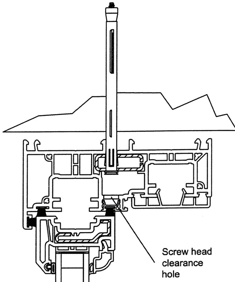
The fixing is achieved using purpose made fixing brackets or through the fixing chamber located in the center of the Outer Frame Profile. If expanding polyurethane foam is used as a gap filler it is recommended that temporary packing be placed between the frame and sashes to maintain the clearance gap whilst the foam cures.
