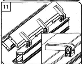
The sash can be removed and fitted when in an open position by lifting or lowering the sash assembly onto the frame datum.
