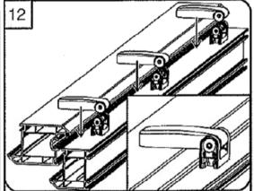
Alternatively the sash can be removed and fitted In the closed position by removing the security screws and hinges pins and then lifting the sash off the frame part.
