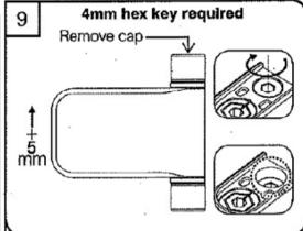
Height adjustment: Using a 4mm hex key turn the screw down to lift the hinge by up to 5mm.
